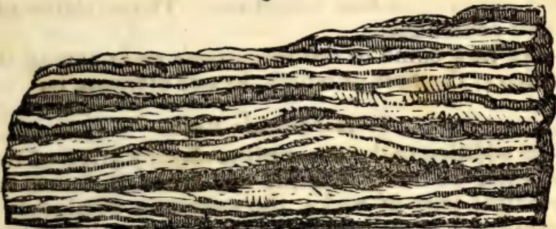
Fragment of gneiss. Section at right angles to planes of stratification.
